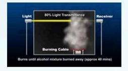
Halogens. To test whether a material is halogen free or not, the tests IEC 60754-1 and 60754-2 are used. The acidity of the gasses from burning materials is measured. Being halogen-free, means that the materials used in the cables do not contain any halogens, such as chlorine, bromine, iodine and fluorine. In order to attain the self-extinguishing effects that halogens have
