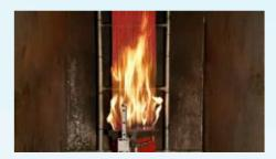
Fire resistance tests are aimed at verifying the circuit integrity behaviour of a cable under fire conditions. The main three different test methods are IEC 60331-21 or IEC 60331-1 or IEC 60331-2, used for power and control cables. Marine cable standards require the IEC 60331-21 test, where the cable sample is subjected to a flame at 750 °C for 90 minutes followed by a 15 minutes cooling period while the rated voltage is being
