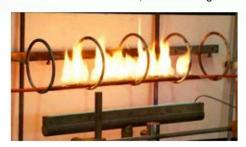
IEC 60331-1 test, or for diameter not exceeding 20 mm IEC 60331-2, in which a bent cable, affected by mechanical shock, is subjected to a 830 °C flame for minimum 90 minutes.
