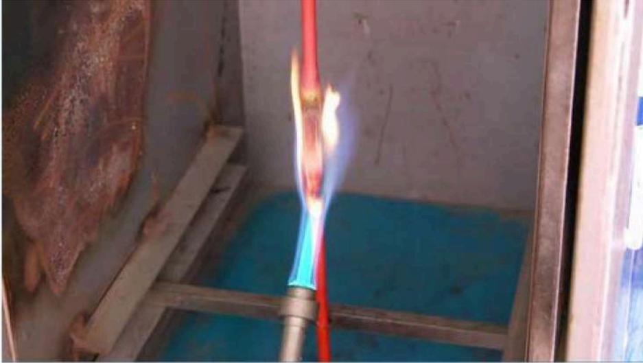
Flame spread is tested on bunched cables in accordance with IEC 60332-3-22, simulating the fire behaviour of the cables installed in a bunch. The main category that is used is A. This is based on an amount of 7 liters of combustible material per meter. The bunch of cables has to be minimum 3.5 m high when it is in a test chamber subjected to fire from a burner directed at the cables for forty minutes. The cable bunch may not burn more than 2.5 m above the burner. Please see figure 2.
