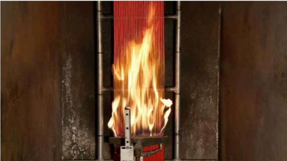
Fire resistance tests are aimed at verifying the circuit integrity behaviour of a cable under fire conditions. The main three different test methods are IEC 60331-21 or IEC 60331-1 or IEC 60331-2, used for power and control cables. Marine cable standards require the IEC 60331-21 test, where the cable sample is subjected to a flame at 750 °C for 90 minutes followed by a 15 minutes cooling period while the rated voltage is being
